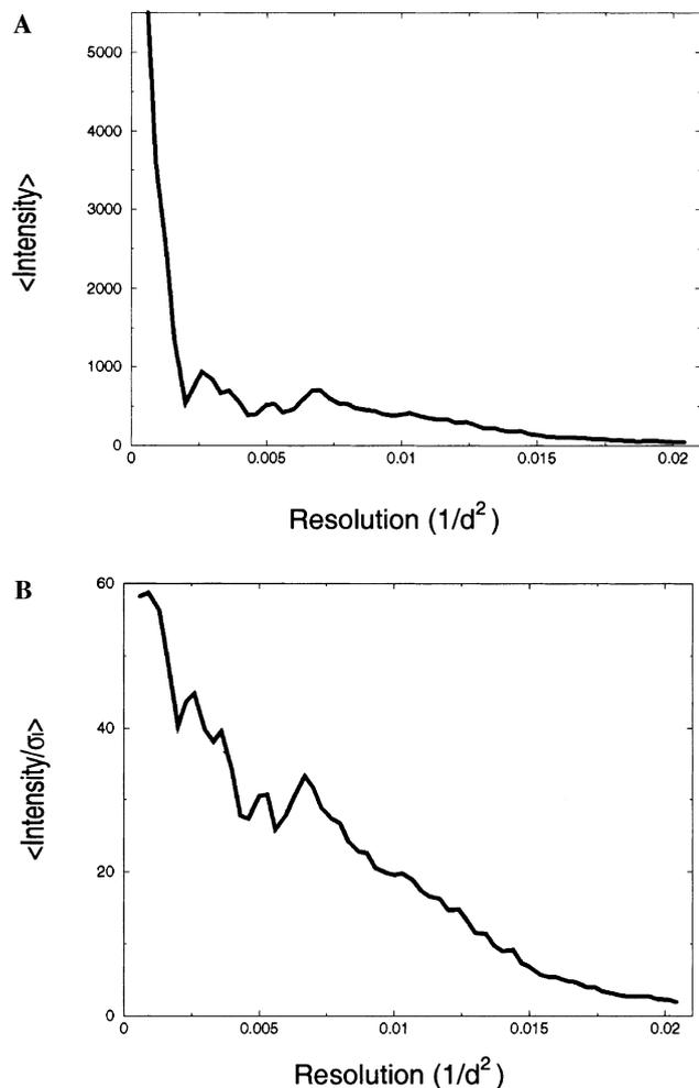
Fig. 4. The mean intensity plotted against resolution for observed X-ray data (A) in the resolution range 60–7 Å ( $1/d^2 \sim 0.0006$ –0.02). (B) The mean distribution of intensity normalized by the standard deviation of the error associated with the measured intensity is plotted versus the resolution ( $1/d^2$ ). At 12-Å resolution the  $I/\sigma_I$  is larger than 12 and it drops to  $\sim 2$  at 7 Å.
