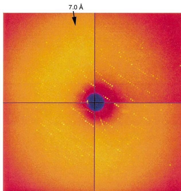
Fig. 3. A diffraction image recorded from bacteriophage P22 portal ring crystal oscillated 0.7° with an exposure time of 30 s. The X-ray wavelength was 1.0  $\text{\AA}$  and the crystal to detector distance was 425 mm. The vertical edge of the image corresponds to a resolution of 4.5  $\text{\AA}$ . Diffraction intensities can be accurately measured including a low resolution of  $\sim 60 \text{\AA}$ .
