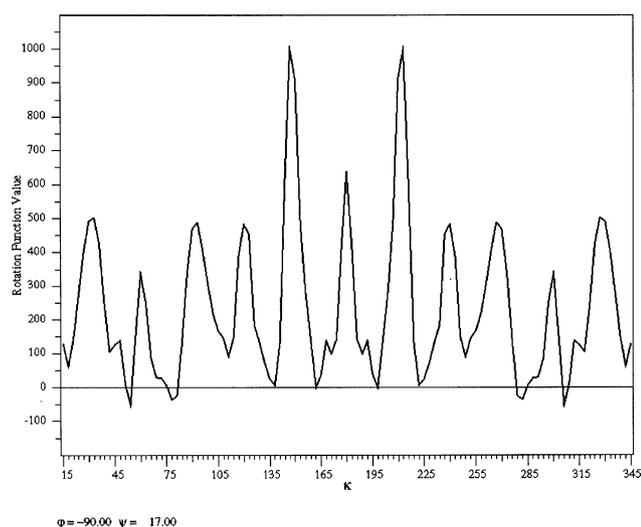
Fig. 6. One-dimensional plot showing the intensity of the rotation function at fixed values of  $\phi = -90^\circ$  and  $\psi = 17^\circ$  and searching  $\kappa$  from  $0^\circ$ – $360^\circ$ . The existence of a 12-fold noncrystallographic axis is suggested by the appearance of a maximum of the rotation function every  $30^\circ$ . The peak at the origin ( $0^\circ = 360^\circ$ ) has been omitted for clarity. Here the rotation function has a maximum value.
