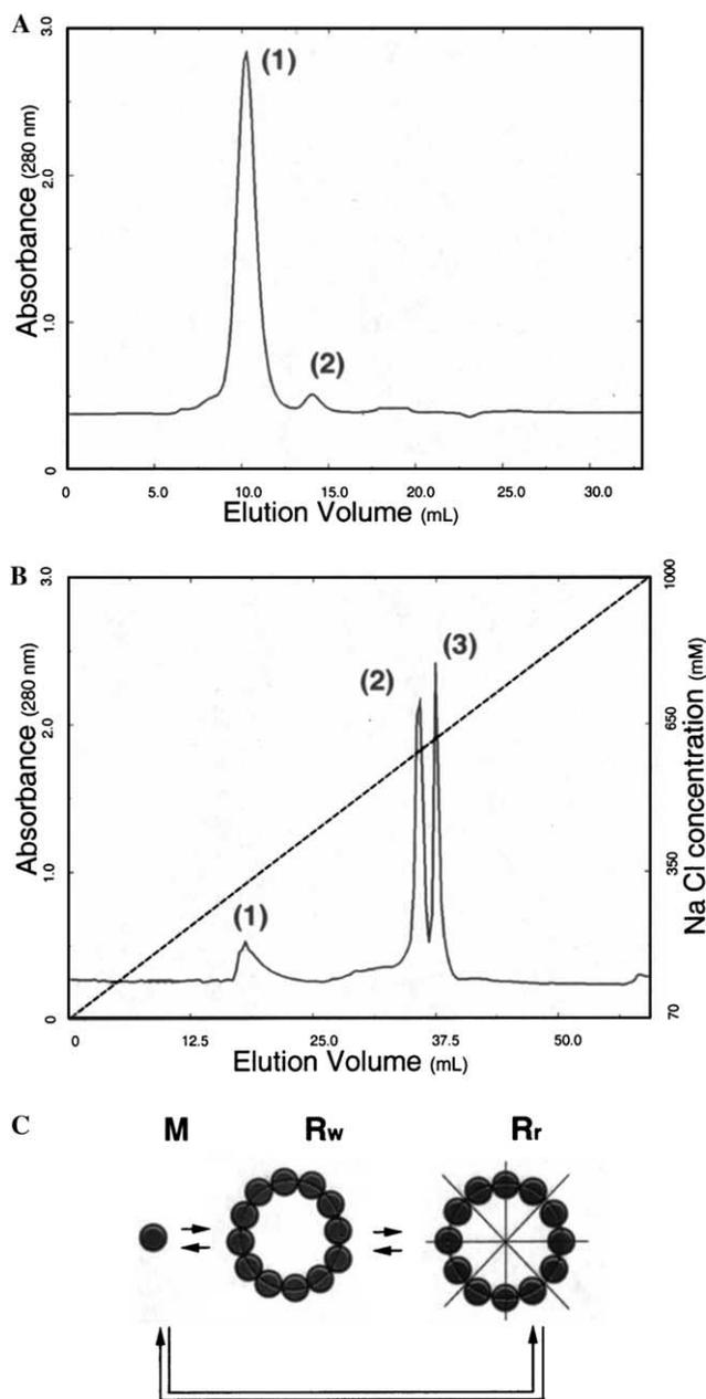
Fig. 1. Dynamic instability of bacteriophage P22 portal rings. (A) Gel filtration chromatogram of purified reassembled portal rings. (B) Separation of different subpopulations by ion-exchange chromatography. (C) Diagram showing the equilibrium existing among portal monomers (M), oligomeric particles formed by the correct number of subunits (R<sub>r</sub>, right ring) and aberrant rings (R<sub>w</sub>, wrong ring).
